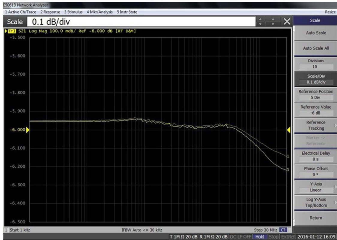
Figure 70: The 6dB splitter is accurate to within 0.25dB across the full frequency range of the instrument.
