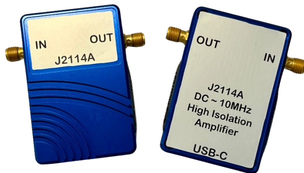
Figure 49: The J2114A is connected like the J2102B in the 2-port shunt-through setup (as close to Port 2 as possible). Inclusion of the transformer eliminates the low frequency distortion caused by instrumentation ground loops.
