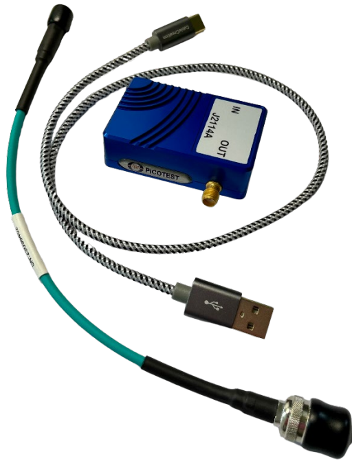
Figure 50: The J2114A is powered by a USB connection and comes with PDN Cable.
