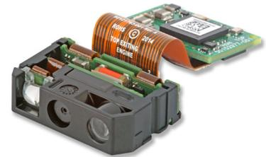
**FIGURE 3. HONEYWELL GEN7 DB WITH THE N3601 SCAN ENGINE**
