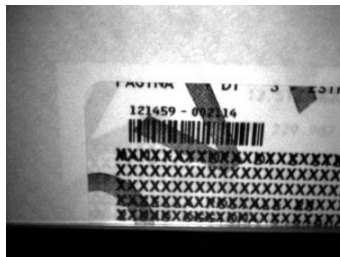
Figure 123. Overprinted Barcode Readable by ABR Through the Envelope Window Film
