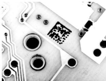
Figure 126. Data Matrix Code Directly Marked on PCB Surface by Using Laser Etching Technology
