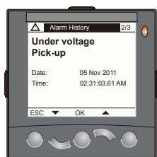
Alarm pick-up and drop-out.
