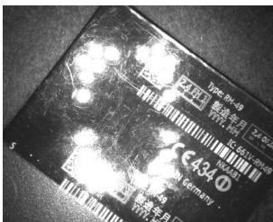
Figure 173. Example A: Incorrect Illumination
