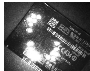
Figure 175. Example C: Good Illumination on Right Code
