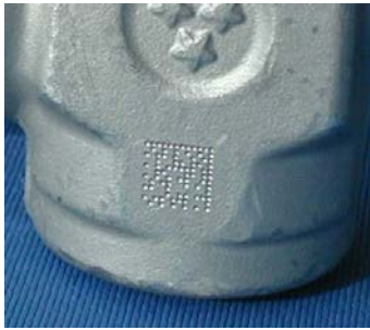
Figure 152. Dot Matrix Code Directly Marked on Metal Surface by Using Dot Peening Technology
