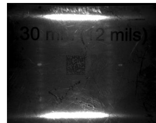
Figure 194. Multicolored DPM - Peripheral Group Top and Bottom Sectors On: Incorrect Illumination
