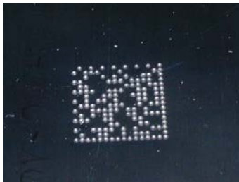
Figure 154. Directly Marked Dot Matrix Code Characterized by Outstanding Separation Distance between Adjacent Code Elements
