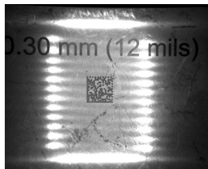
Figure 193. Multicolored DPM - Peripheral Group ALL Sectors On: Suboptimal Illumination
