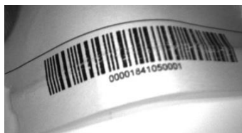
Figure 151. Barcode Printed on Curved Surface Readable by ABR in spite of Image Optical Distortion
