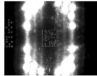
Figure 186. Multicolored DPM - Central Group: Incorrect Illumination
