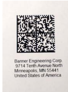
Figure 148. Address Coded in Data Matrix Symbology for Automated Mail Processing
