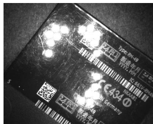
Figure 174. Example B: Good Illumination on Left Code
