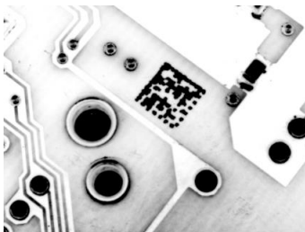
Figure 156. Data Matrix Code Directly Marked on PCB Surface by Using Laser Etching Technology
