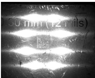
Figure 192. Red: Incorrect Illumination
