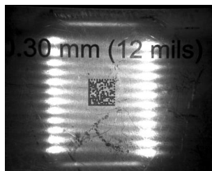
Figure 195. Multicolored DPM - Peripheral Group Left and Right Sectors ON: Good Illumination
