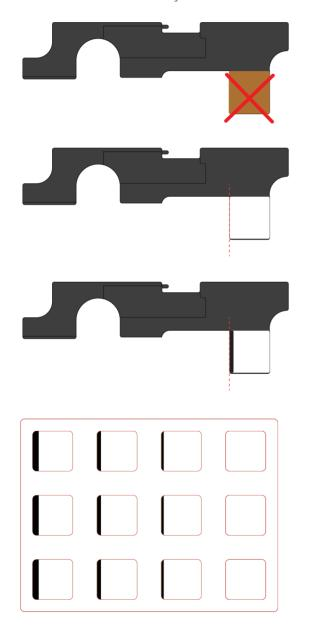
Remove the original copper sheet on the selector plate (if not, it may affect the senor to detect)
