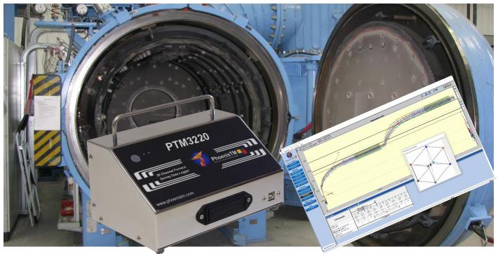
At PhoenixTM we believe that Data Loggers for furnace surveying must be built to operate in harsh environments while maintaining high accuracy throughout their operating temperature range. The PTM 3210 (10 channel) and PTM 3220 (20 Channel) Data Loggers include these key features:
