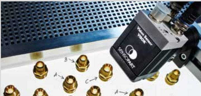
**The one with a BLOB:** With the new BLOB detector (Binary Large Object), the VISOR® detects even small differences between objects, counts parts or detects whether a part is face up or face down.
