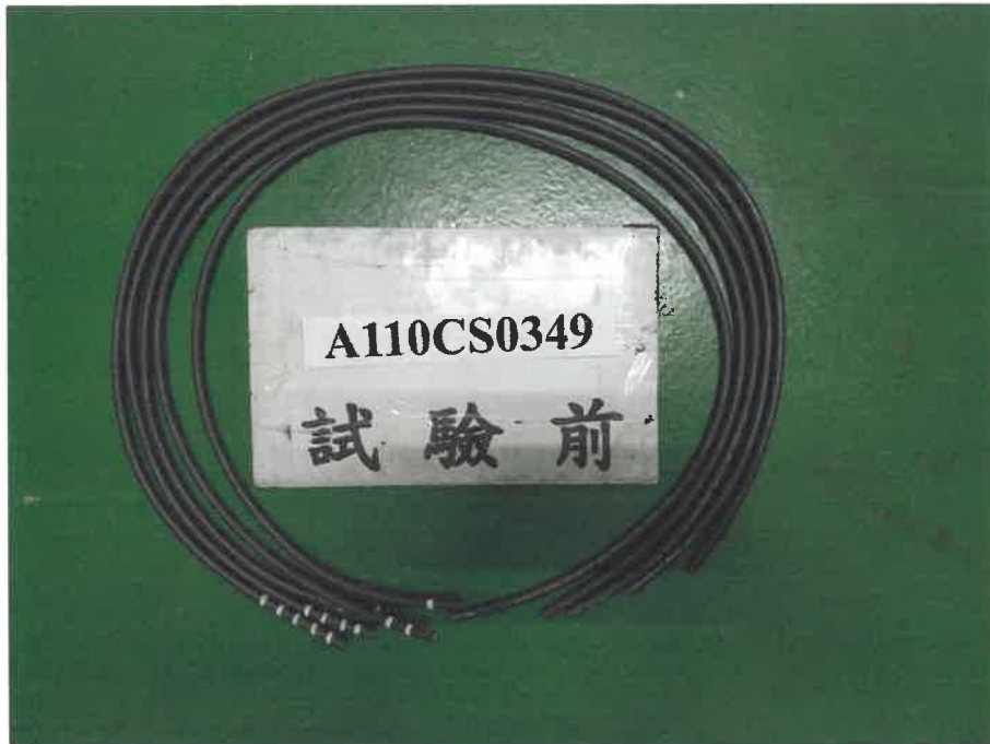
The sample condition before burnt
