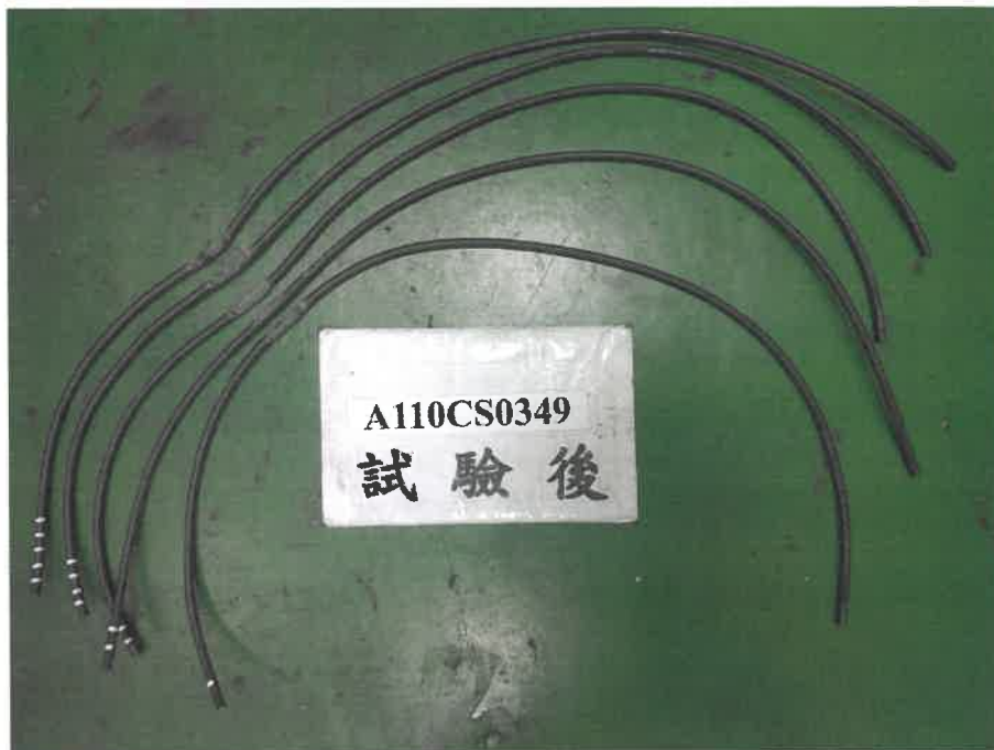
The sample condition after burnt
