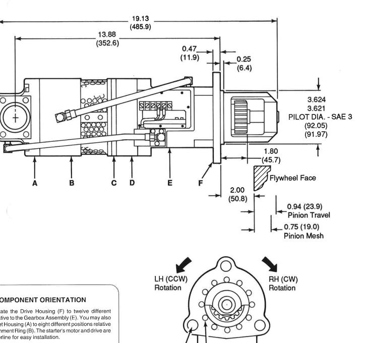
Three 0.66 (16.76) dia. holes equally spaced on a 5.75 (146.1) DBC for SAE 3 mounting.
