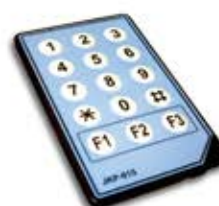
JKP-015 (keypad unit) 90(L)× 55(W)×8(H)mm
