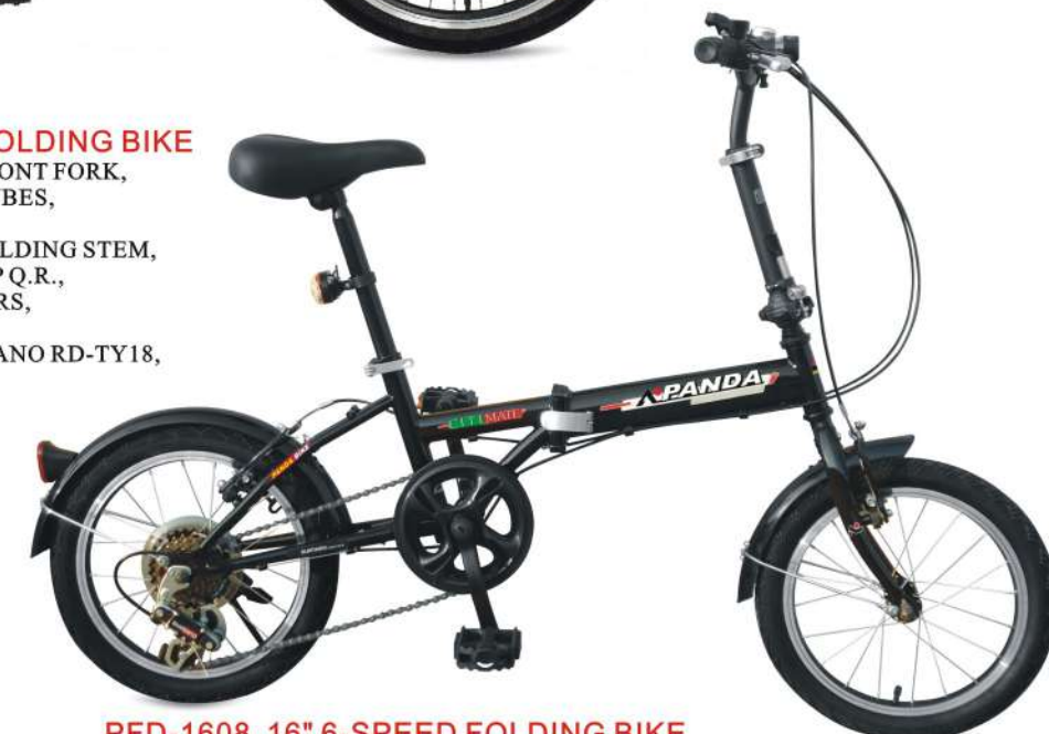
PFD-1608 16" 6-SPEED FOLDING BIKE 16" STEEL FRAME & FRONT FORK, 16" x 1.75 BLACK TIRES, BUTYL TUBES, STEEL HUBS, ALLOY RIMS, STEEL V-BRAKE, ALLOY HANDLEBAR, STEEL FOLDING STEM, ALLOY QUICK RELEASE, SHIMANO TY-18SS SL-TZ20 6 SPEED INDEX DERAILLEUR.
