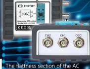
CTR gained via an FRA can be measured through M352XA as well. We call it the equivalent ΔCTR.
