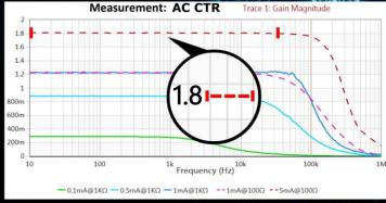
The F1 example was made via the J2200A, M352XA, and the OMICRON Lab Bode 100 VNA.
