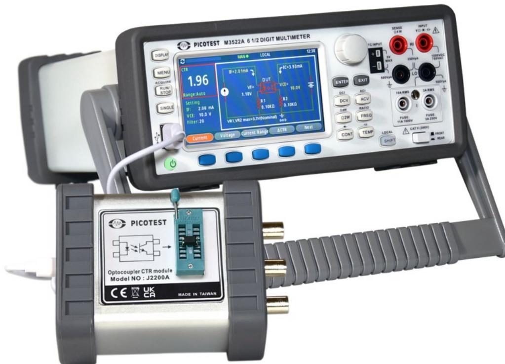
**Fig. 4 - Measurement Setup with J2200A and M3522A.**
