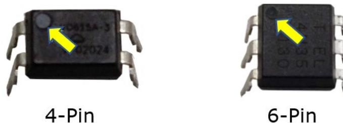
**Fig. 2 - Depiction of 4-pin and 6-pin Optocoupler Packages.**
