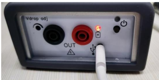
Figure 3 : J2122A with red light, during charging
