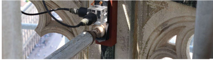
Figure 2: High sensitivity ICP® accelerometers in use - low frequency and seismic.
